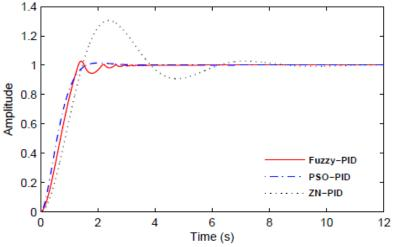
Fig. 5. Response of system for fuzzy, PSO-PID and PID controllers.
