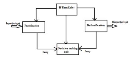
Fig. 2. Block diagram of fuzzy logic.
