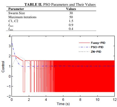
Fig. 6. Control efforts of system for fuzzy, PSO-PID and PID controller.
