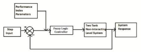
Fig. 3. Fuzzy controller for two tank non-interacting system.
